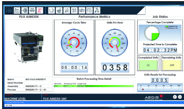
FactoryLogix IIot/MES manufacturing intelligence dashboard for Fuji AIMEX III.
